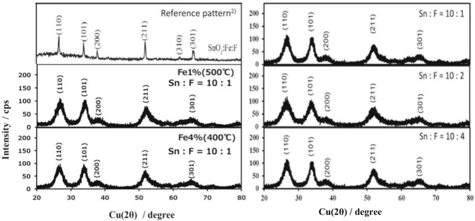
**Fig. 1** (left hand) XRD patterns of FTO doped with 4% Fe and 1% Fe annealed at 400 °C and 500 °C, respectively, and (right hand) XRD of 1% Fe doped FTO with the mole ratios of Sn:F = 10:1, 10:2 and 10:4, annealed at 400 °C for 2 h.
