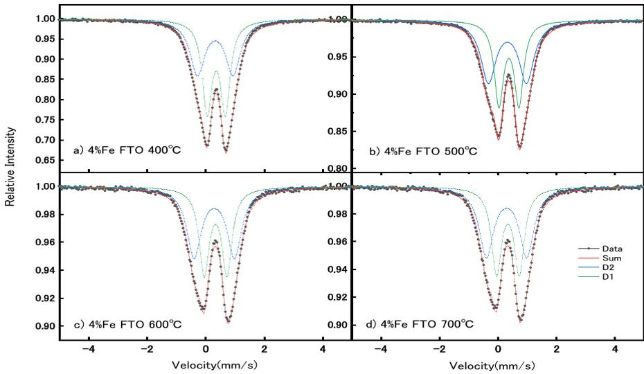
**Fig. 4** Mössbauer spectra of 4% Fe doped FTO annealed at various temperatures
