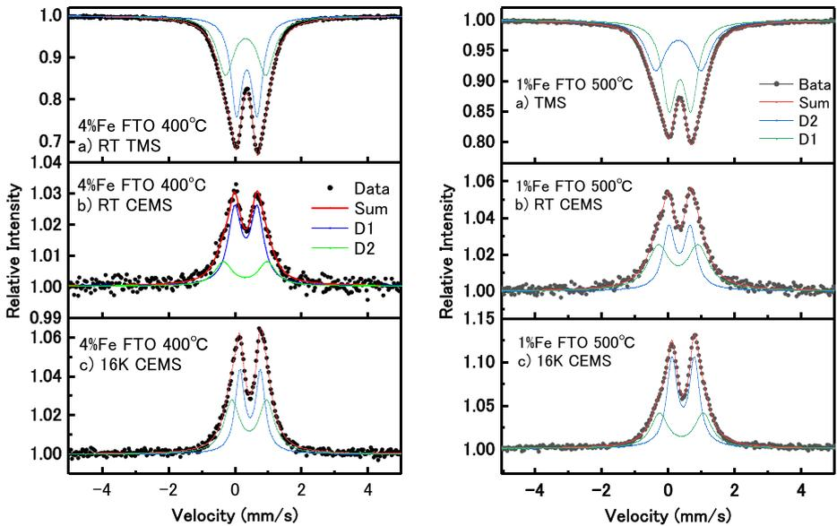
**Fig. 6** Transmission and conversion Mössbauer spectra (TMS and CEMS) of 4% Fe doped FTO annealed at 400 °C and 1% Fe doped FTO annealed at 500 °C, respectively
