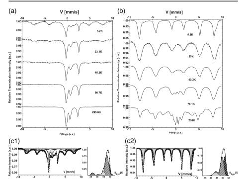
Fig. 2 The experimental Mössbauer spectra of the sample VS-3 (a) and VS-3m (b) for  $T \in 296K-5K$ , and the fit of LHeT magnetic field distribution (c1) and (c2) respectively
