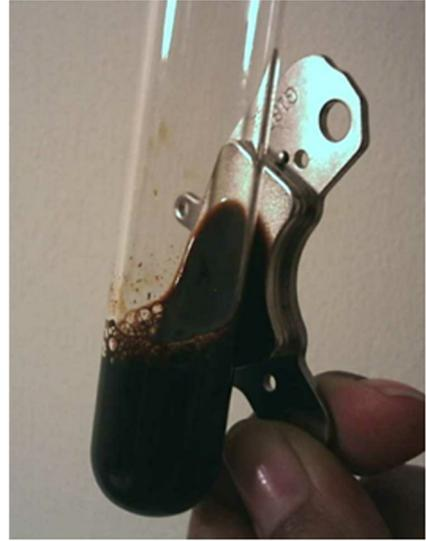
for 2 hours. The etching of the substrates with the KOH solution was implemented locking for a well bonding between the surface charge of the magnetic nanoparticles and  $\text{SiOH}_2^+$  groups present in the surface of the glass substrate for the concentration of KOH employed.
