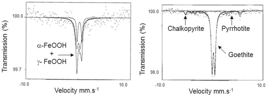
**Fig. 6** Mössbauer spectra of (left) froth and (right) final leachate products remaining in the leaching of a Ni-Cu-Co-sulphide
