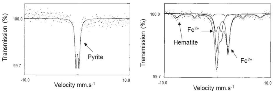
**Fig. 5** Mössbauer spectra of (*left*) coal containing only pyrite used for gasification and (*right*) the final ash product formed after gasification, containing a  $\text{Fe}^{2+,3+}$ -glass and hematite
