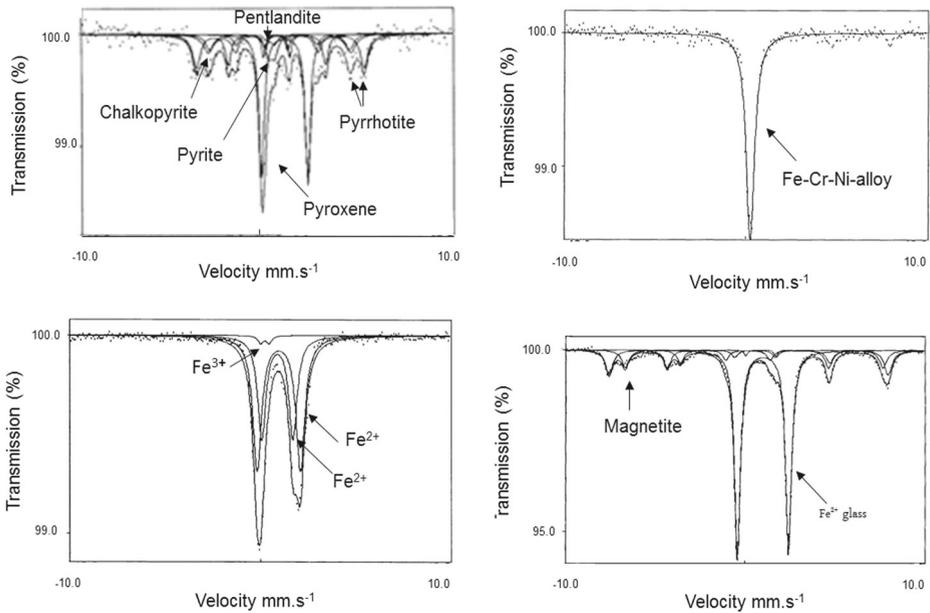
**Fig. 7** Mössbauer spectrum of an ore sample (*top left*) found in the Bushveld Igneous complex and the spectrum of the Fe-Cr-Ni-alloy formed in the electric furnace (*top right*). The spectrum of the electric furnace slag showing a high  $Fe^{2+}/Fe^{3+}$  ratio (*bottom left*) and the spectrum of the slag from the slag-cleaning furnace and in the bottom right showing magnetite and almost no  $Fe^{3+}$  indicating minimal loss of Ni
