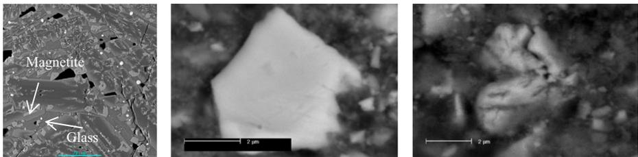
**Fig. 8** On the left a backscattered electron image of the slag containing magnetite [23]. On the right an euhedral chalcopyrite particle (*left*) and a pentlandite particle (*right*) after leaching, showing almost complete dissolution of the latter [23]
