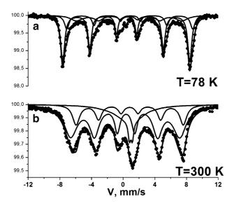
Fig. 2 Mössbauer spectra of 25 nm nanoparticles measured at 78 K and 300 K
