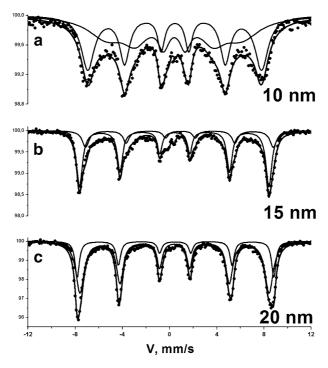
Fig. 1 Mössbauer spectra of 10-25 nm nanoparticles measured at 78 K
