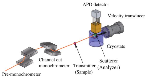
**Fig. 1** Schematic of experimental setup. The glancing angle of the incident radiation with respect to the surface of the scatterer is approximately  $7^\circ$  and delayed emission from the irradiated surface of the scatterer was measured using a multielement Si-APD detector ( $4 \times 2$  APDs elements, with a detection area of  $3 \times 5 \text{ mm}^2$  each)
