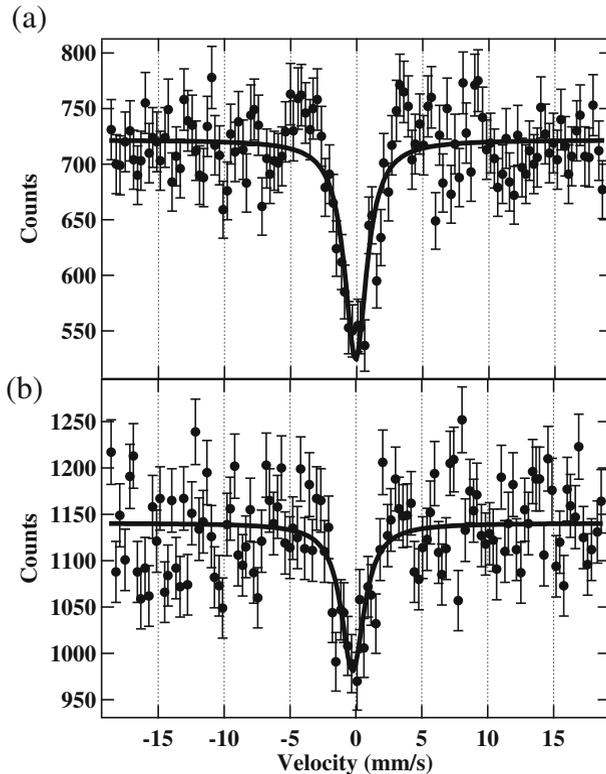
**Fig. 2**  $^{125}\text{Te}$  Mössbauer spectra measured by using SR. As a transmitter,  $\text{Mg}_3\text{TeO}_6$  with a thickness of  $5.0 \text{ mg } ^{125}\text{Te} / \text{cm}^2$  was used at 300 K. As a scatterer,  $\text{Mg}_3\text{TeO}_6$  with a thickness of  $0.5 \text{ mg } ^{125}\text{Te} / \text{cm}^2$  was used at **a** 60 and **b** 300 K. The *solid line* shows fit spectra with Lorentzian line shapes
