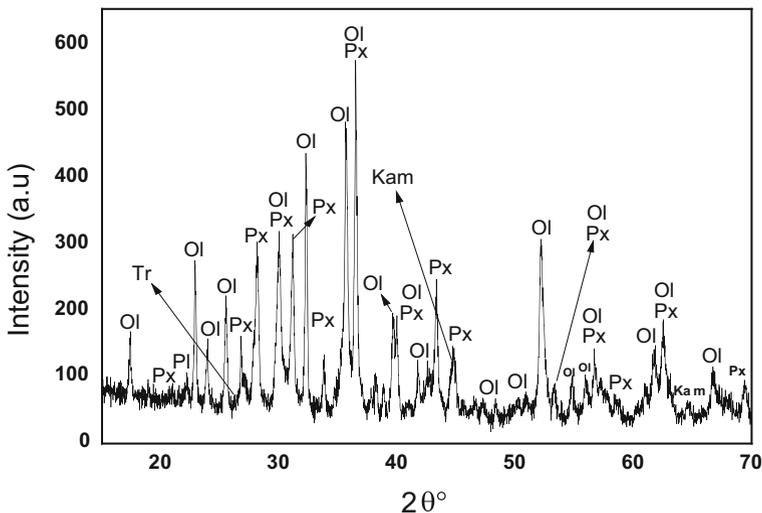
**Fig. 2** X-Ray diffraction patterns for mineral phases in the Aba panu meteorite samples, olivine, pyroxene, troilite, and kamacite, phases, with the decreasing in order of abundance
