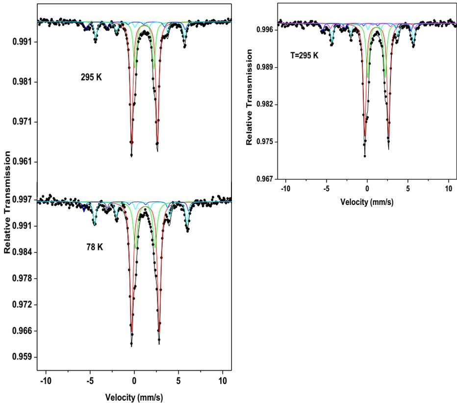
**Fig. 3** (left) Mossbauer spectra of the Aba panu meteorite with indicated temperatures, (right) The 295 K Mossbauer spectrum of New Halfa meteorite for comparison [11]
