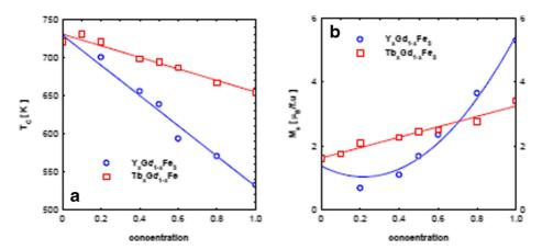
Fig. 2 Values of the (a) Curie temperature; **b** saturation magnetic moment of  $R_xGd_{1-x}Fe_3$  series as function of x parameter for R concentration (R = Tb, Y)
