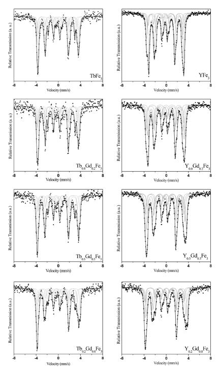
Fig. 3 Room temperature  $^{57}$ Fe Mössbauer effect spectra of the selected  $R_xGd_{1-x}Fe_3$  (R = Tb,Y) intermetallics
