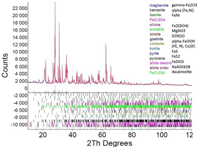
**Fig. 2** XRD pattern obtained at RT of the NWAXX meteorite
