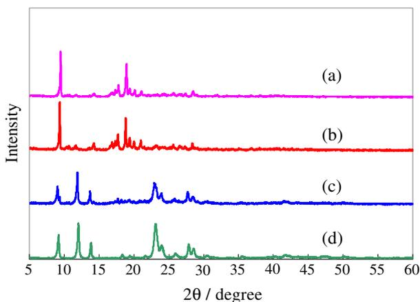
**Fig. 2** Powder X-ray diffraction patterns of **a**  $\text{Fe}(\text{NCS})_2\text{bpp}_2$  (simulation), **b**  $\text{Fe}_{0.14}\text{Zn}_{0.17}\text{Co}_{0.69}(\text{NCS})_2\text{bpp}_2$  (red crystals), **c**  $\text{Fe}_{0.20}\text{Zn}_{0.63}\text{Co}_{0.17}(\text{NCS})_2\text{bpp}$  (blue crystals), and **d**  $\text{Zn}(\text{NCS})_2\text{bpp}$
