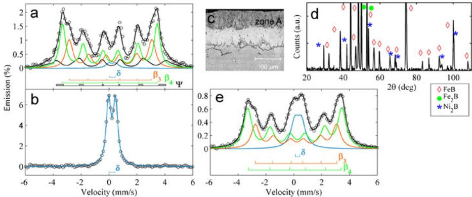
**Fig. 1** CXMS for  $\text{Fe}_{64}\text{Ni}_{36}$  borided for **a** 20 min and **b** 1 h. **c** metallographic cross-section and **d** XRD for the 8h-borided  $\text{Fe}_{64}\text{Ni}_{36}$ , **e** CXMS for the same sample after 450  $\mu\text{m}$  surface abrasion
