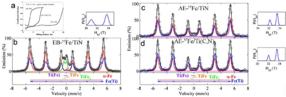
**Fig. 2** **a** friction curves measured for EB-, AE-TiN, AE-Ti(C,N); **b, c, d** CEMS spectra for EB-<sup>57</sup>Fe/TiN, AE-<sup>57</sup>Fe/TiN, AE-<sup>57</sup>Fe/Ti(C, N) respectively
