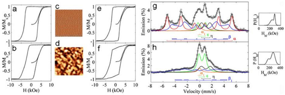
**Fig. 3** Polar loops and  $1 \mu\text{m}^2$  AFM for **a–c** FePt(15) and **b–d** FePt(20) respectively. Polar loops and CEMS spectra respectively for **e–g** FePt(15)/Fe(7) and **f–h** FePt(20)/Fe(7)
