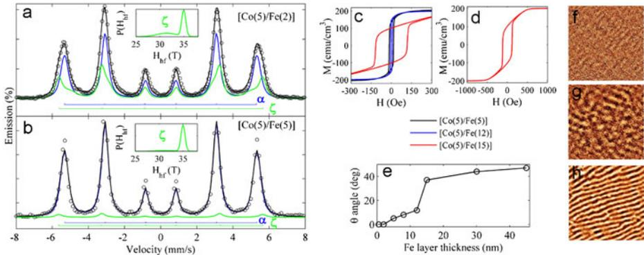
**Fig. 4** CEMS spectra for **a** [Co(5)/Fe(2)] and **b** [Co(5)/Fe(5)], AGFM loops for **c** [Co(5)/Fe( $t_{Fe}$ )] ( $t_{Fe} = 5, 12, 15$  nm) and **d** [Co(5)/Fe(15)], **e** angle between the magnetization vector and the film plane vs. the Fe layer thickness, MFM images for **f** [Co(5)/Fe(5)], **g** [Co(5)/Fe(12)] and **h** [Co(5)/Fe(15)]
