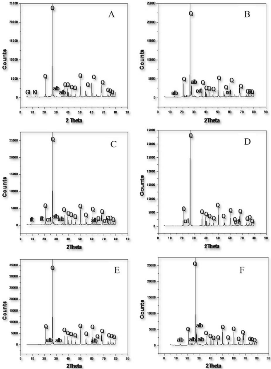
**Fig. 3** XRD spectra of **a** (blackish), **b** (greenish), **c** (greyish), **d** (reddish), **e** (whitish), **f** (yellowish) sandstones showing the minerals identified (Q = quartz, alb = albite, Gl = Glauconite, KI = kaolinite, ort = orthoclase, ilt = illite and crl=crsobilite)
