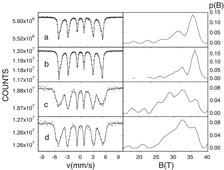
**Fig. 2** Typical room temperature  $^{57}\text{Fe}$  Mössbauer spectra and the corresponding hyperfine field distributions of different origin TaC containing ball milled steel powders **a** VVER+ commercial TaC, **b** VVER+ home made TaC, **c** EUROFER+ commercial TaC and **d** EUROFER+ home made TaC
