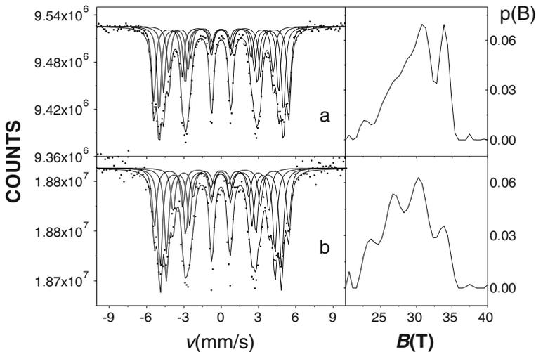
**Fig. 3**  $^{57}\text{Fe}$  Mössbauer spectra (decomposed into four sextets) and hyperfine field distributions of pure EUROFER ball milled steel **a** and its state after mechanical alloying with commercial TaC **b**
