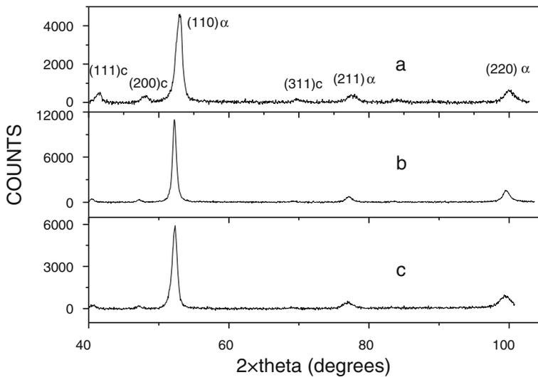
**Fig. 1** XRD patterns of the ball milled steel powders **a** VVER+TaC, **b** VVER+NbC, **c** EUROFER+NbC
