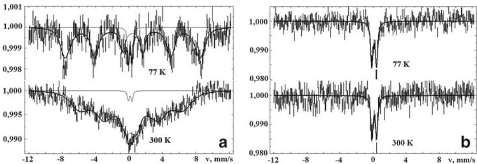
**Fig. 2**  $^{57}\text{Fe}$  Mössbauer spectra for initial NP (**a**) and a rat brain in 3 months after the NP injection (**b**). The results of simultaneous treating are represented by *solid lines*. These are partial relaxation spectra of NP, additional non relaxation doublet as well as the resulting spectra
