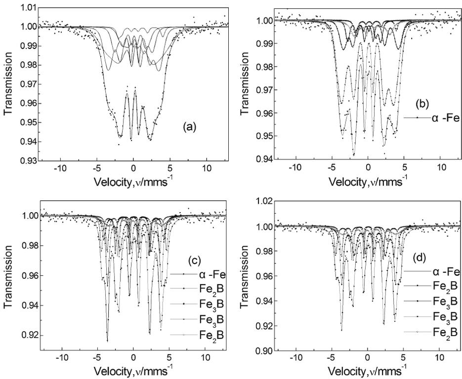
**Fig. 3** Mössbauer spectra of Fe-B-P particles (a) as-prepared, (b) annealed at 300°C, (c) 400°C, (d) 500°C
