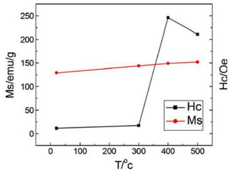
shown in Fig. 4. The coercivity of the sample after annealing at 400 °C and 500 °C has further increased and this leads to a deterioration of the magnetic properties of the samples because the crystallized phases block domain wall motion. The results show that the soft magnetism of samples with trace crystallization is slightly improved by the annealing treatment. But the soft magnetism of completely crystallized samples has deteriorated.
