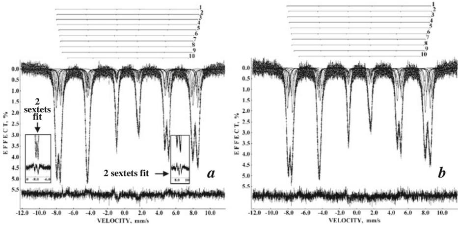
**Fig. 3** Mössbauer spectra of the NA (a) and NB (b) samples measured in 4096 channels at  $T = 295$  K. 1–10 are the components obtained by the appropriate fit. The differential spectra are shown below
