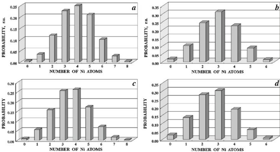
**Fig. 4** Histograms of probabilities of various numbers of  $\text{Ni}^{2+}$  in local microenvironment of the  $^{57}\text{Fe}$  in the tetrahedral (a, c) and octahedral (b, d) sites within the sphere of 3.5 Å radius in  $\text{NiFe}_2\text{O}_4$  nanoparticles: the NA (a, b) and NB (c, d) samples
