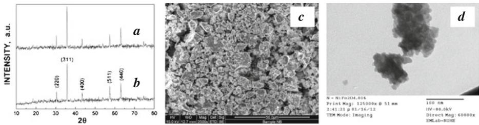
**Fig. 1** X-ray diffraction patterns of the NB (a) and NA (b) samples, SEM (c) and TEM (d) images of the NB sample
