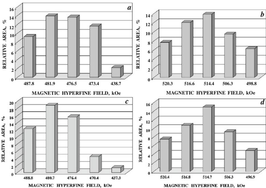
**Fig. 5** Histograms of the relative areas of magnetic sextets related to the <sup>57</sup>Fe in the tetrahedral (**a**, **c**) and octahedral (**b**, **d**) sites for the fit of Mössbauer spectra of the NA (**a**, **b**) and NB (**c**, **d**) samples using ten magnetic sextets
