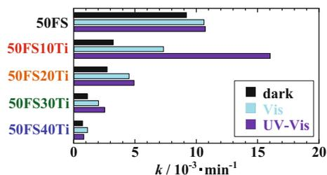
red square). Moreover, all samples except for 50FS10Ti have no clear difference in the absorbance under the visible light irradiation and that under the UV-visible light irradiation. These results show that annealed 50FS10Ti exhibited photocatalytic effect not only under visible light irradiation but also under UV-visible light irradiation. It is concluded that annealed 50FS10Ti glass has the practical photocatalytic effect which is responsive to both visible and UV lights.
