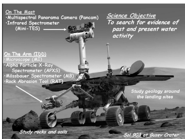
Fig.1 : Artist view of the Mars Exploration Rovers. Size of the rover is about 1m x 1m (length and width) by ~1.6m high (position of the Panorama Camera).
